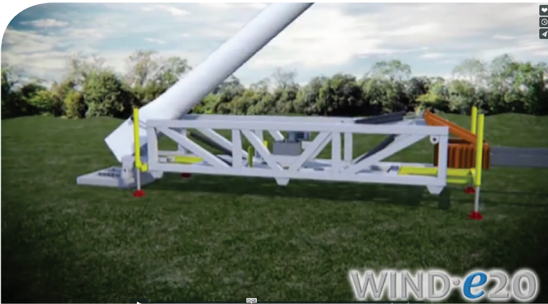
The transport carriage also doubles as an erection mechanism that tilts the turbine onto its prepared foundation.
